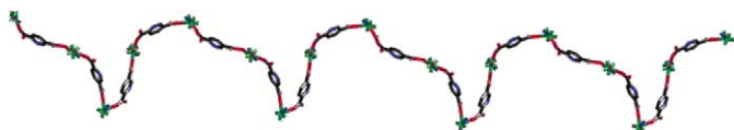
Fig. 3. The helical chains in the three-ply layer. For clarity, only Cd centers and nicotinate ligands are shown.
